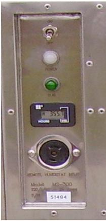
A "POWER ON" lamp is provided to indicate that power is applied to the machine.
