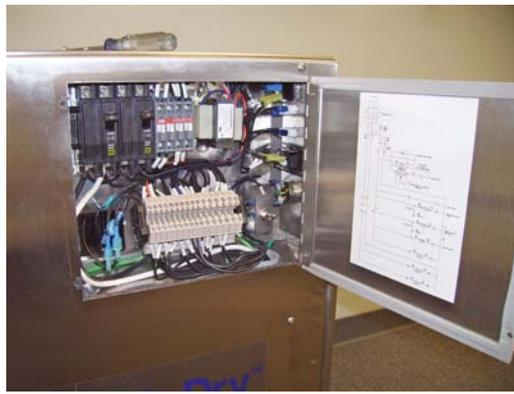
The controls in this machine are UL listed and provide for automatic operation and all required protection of the machine components. Access to the control panel is via a hinged access cover.
