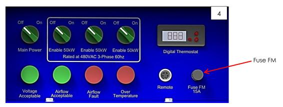
4. To replace fuse FM, locate the fuse holder cap on the far right of the switch panel. Turn the fuse holder cap counter-clockwise and pull the cap with the fuse attach out of the panel. Replace the fuse with an identical 15A fuse (MMC Part #EC-9500-1971). After the fuse has been replaced, insert the fuse cap into the appropriate hole and twist clockwise to lock in place.
