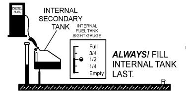
Figure 35. Filling Secondary Internal Fuel Tank
