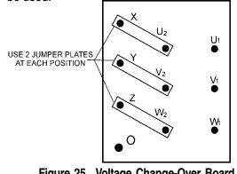
Figure 25. Voltage Change-Over Board 480V Configuration
