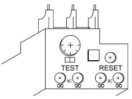
Figure 13. Over Current Relay
