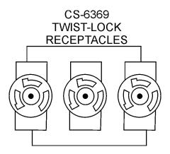
Figure 10. 240/139 VAC Twist-Lock Auxiliary Receptacles
