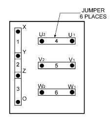
Figure 15. Voltage Change-Over Board 240V Configuration
