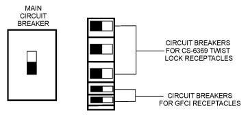
Figure 67. Main, Aux. and GFCI Circuit Breakers (OFF)
