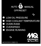
During cranking cycle. The MPEC will attempt to crank the engine for 10 seconds before disengaging. If the engine does not engage (start) by the third attempt, the engine will be shutdown by the engine controller's " Over Crank Protection" mode. If the engine engages at a speed (RPM's) that is not safe, the controller will shutdown the engine by initializing the "Over Speed Protection" mode.
