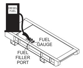
Figure 31. Skid Type Fuel Tank System
