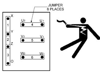
Figure 14. Voltage Change-Over Board 240V Configuration
