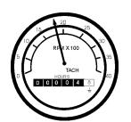
Figure 54. Engine Tachometer Gauge
