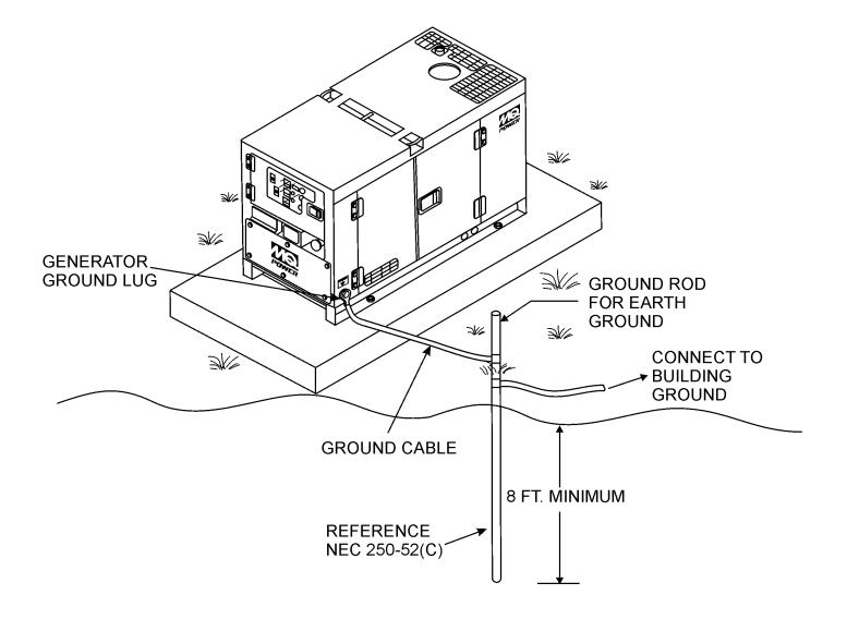
Figure 4. Typical Generator Grounding Application
