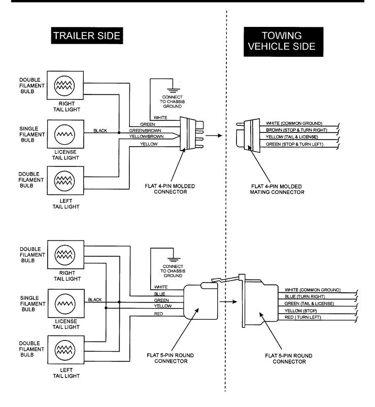
Figure 77. Trailer/Towing Vehicle Wiring Diagram
