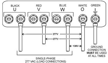
Figure 28. UVWO Terminal Lugs 1Ø-277V Connections
