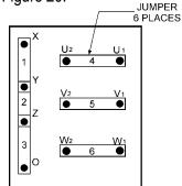
Figure 20. Voltage Change-Over Board 240V Configuration
