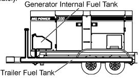
Figure 30. Double Fuel Tank System
