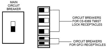
Figure 42. Main, Aux. and GFCI Circuit Breakers (OFF)
