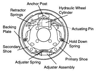
Figure 74. Hydraulic Brake Components
