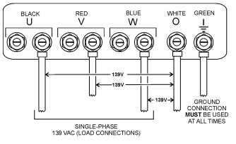
Figure 24. UVWO Terminal Lugs 1Ø-139V Connections
