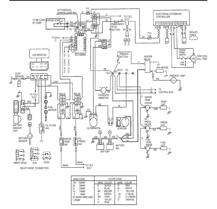
Figure 81. Engine Wiring Diagram (S/N 3701674 and Above)
