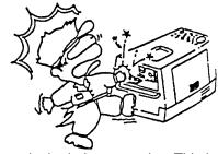
■ **NEVER** touch output terminals during operation. This is extremely dangerous. Always stop the machine when contact with the output terminals.
