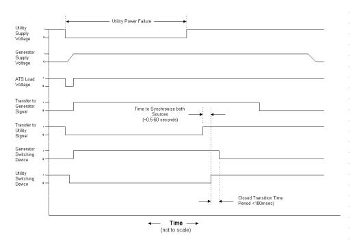
The following operating sequences and time delays are associated with closed transition type transfer switches which momentarily parallel two sources of supply for less than 100 milliseconds. For closed transition type transfer switches, which utilize extended parallel operation for soft-loading operating sequences, refer to separate instruction manual.
