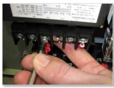
7. Install the extra screw back onto the old PT location and tighten.
