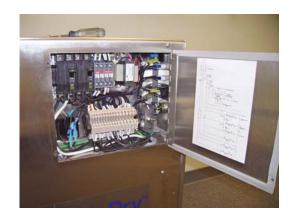
The controls in this machine are UL listed and provide for automatic operation and all required protection of the machine components. Access to the control panel is via a hinged access cover.
