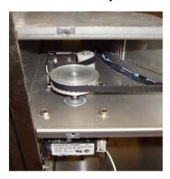
The rotor drive system consists of a fractional hp gear motor, timing pulley, timing belt, and spring tensioner. The gear motor is sealed and permanently lubricated. Check the motor fasteners and timing pulley to be secure. Inspect the timing belt for cracks, tears, or abrasion. The tensioner should keep slack form the belt with light tension.
